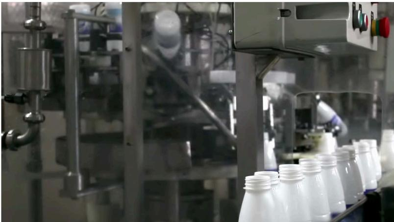
At the plant, milk is tested, homogenized and pasteurized.
