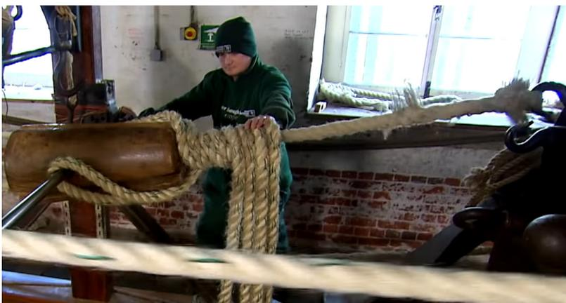
This holds them in place as the rope-making machine twists the three strands into one.
