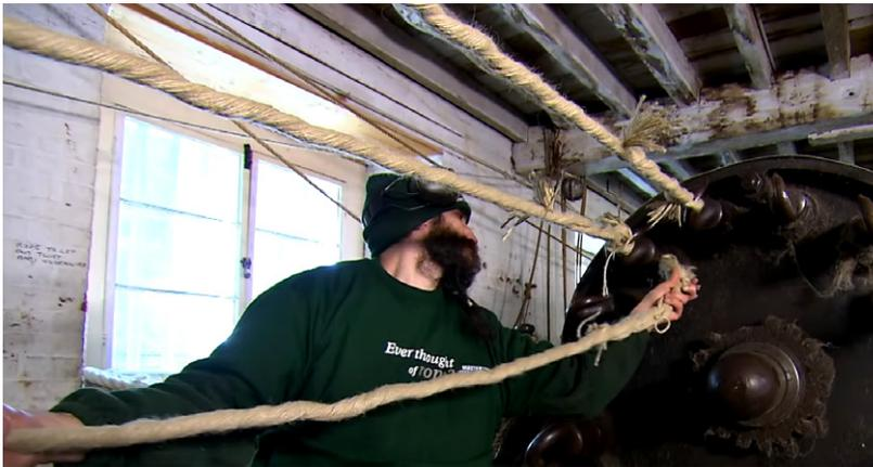
On one side, they tie three of the strands to a machine that will transform them into a rope.
