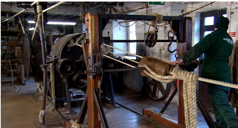
When the cart arrives at the opposite side of the building the rope is formed.
