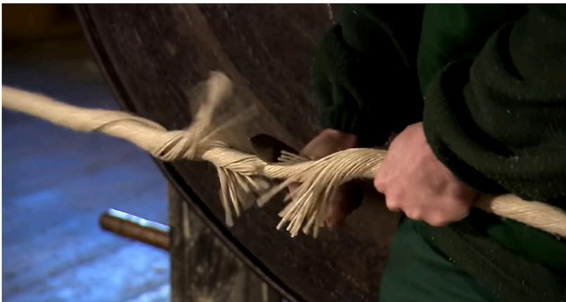
When the machine reaches the back wall, it stops, and workers cut both ends of the strands.
