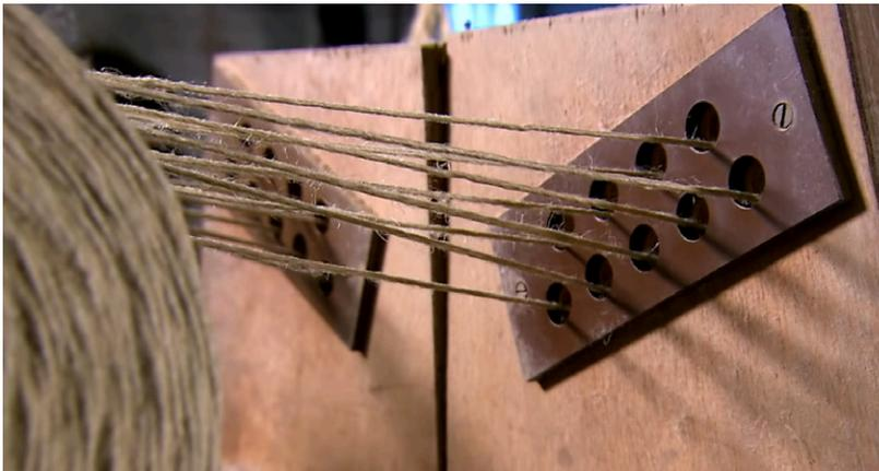
The yarns are funneled through separators which configure them to twist evenly together.
